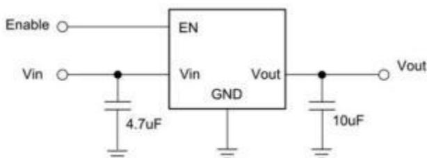
Note: Recommended  $C_{in}$ : 4.7µF/6.3V, Recommended  $C_{out}$ : 10µF/6.3V; Add more capacitance can decrease the ripple.
