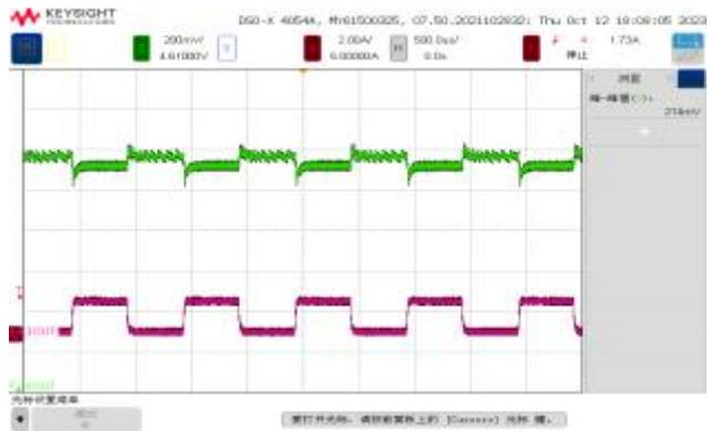
Load dynamic response,  $V_{OUT} = 5V$  ,  $I_{OUT} = 1.5A \rightarrow 3A$
