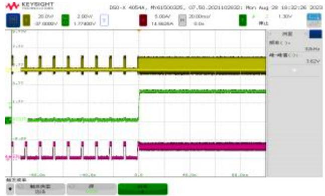
The test conditions are  $V_{IN} = 12V$ ,  $V_{OUT} = 1.0V$ , with external capacitors  $C_{IN}=2 \times 10\mu F$ ,  $C_{OUT} = 2 \times 47\mu F$ , and a temperature of  $T_A = 25. C$ , unless otherwise noted.
