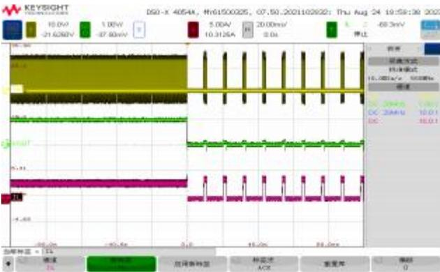
Short-circuit recovery,  $V_{IN}=12V$  ,  $V_{OUT}=1.0V$  Short to 3A
