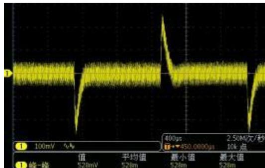
Output the waveform of start-up delay time
