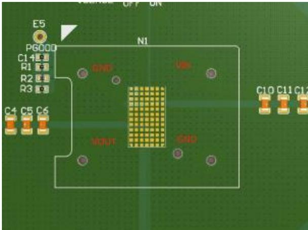
1. Place the **R<sub>FB</sub>** resistor as close as possible to its corresponding pin.
